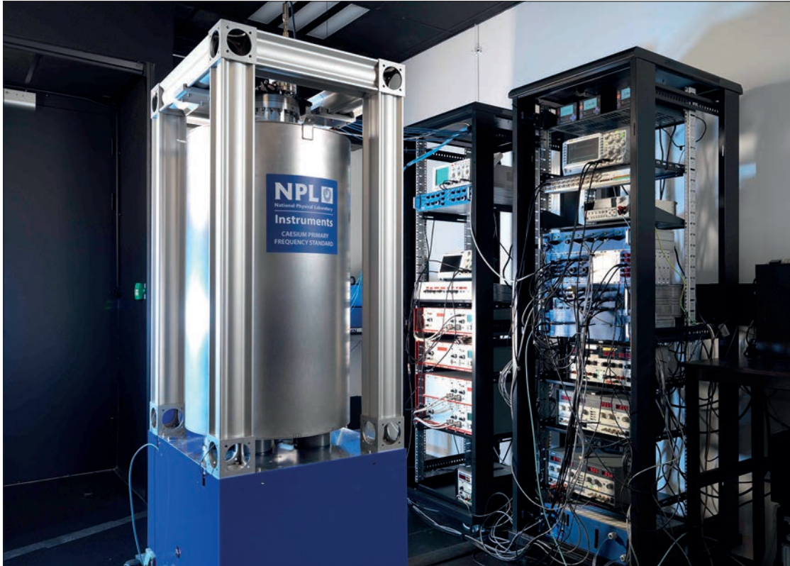
A state-of-the-art NPL Instruments caesium primary frequency standard, next to its control and test electronics © National Physical Laboratory
