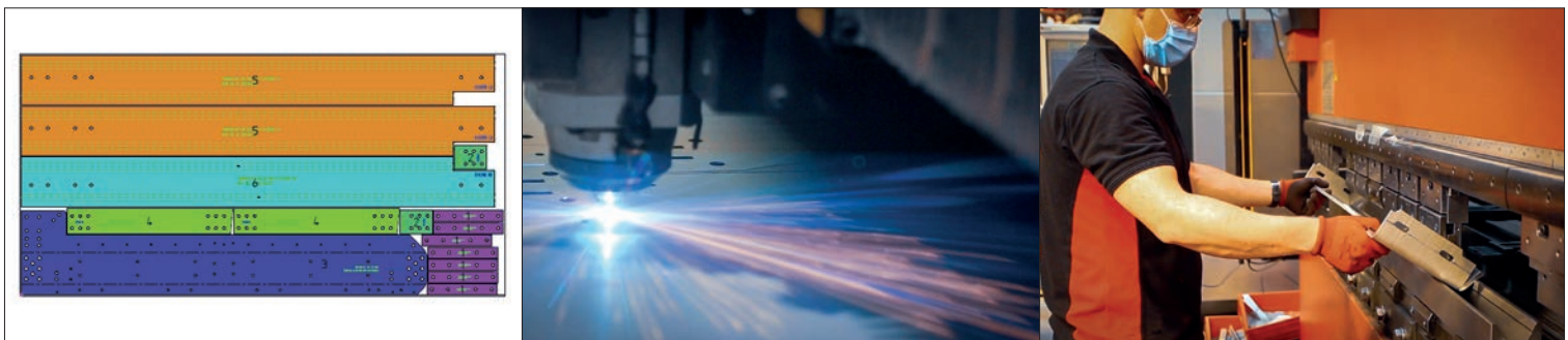
Manufacturing the AVA Bridge (L-R): The computer screen shows a 3 metre by 1.5 metre steel sheet marked up multiple parts to be laser cut, using 92.9% of the sheet, resulting in less wastage and carbon emissions. The sheet is cut by the computer-controlled laser and then folded © X-Treme Systems
