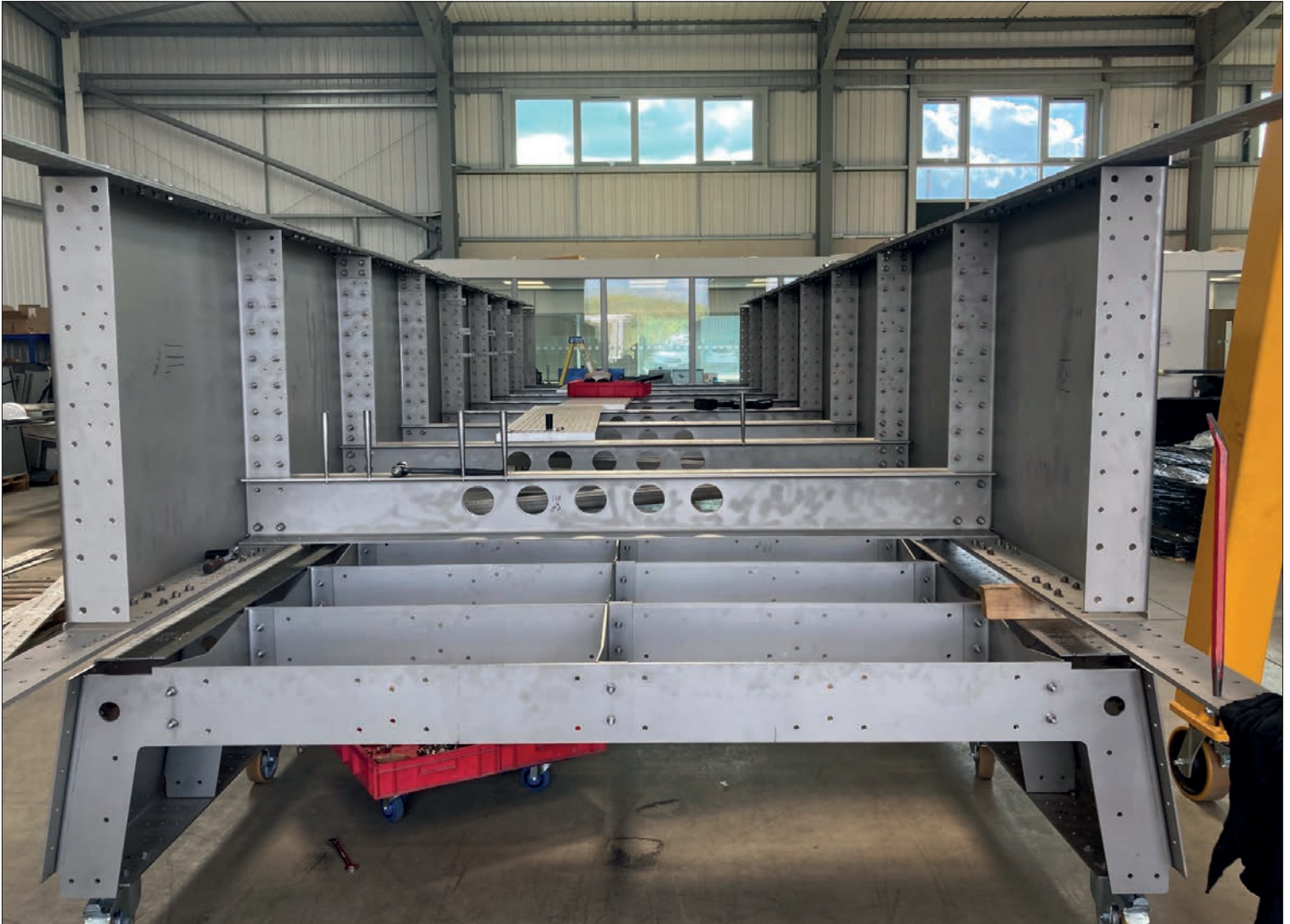
Modifications made following testing of the prototype resulted in the primary structure of a U-frame formed from two longitudinal girders, concealed within the parapet and linked by crossbeams. The main girders are made of 1.2 metre-long panels folded to make a C, with the top and bottom flanges strengthened by extra plates, and all elements bolted together to form a continuous structure. This allowed a continuous glass window to be provided above the parapet, improving the user experience. (The U-frame above is supported on an improvised construction trolley, made from recycled parts of the original prototype) © X-Treme Systems
