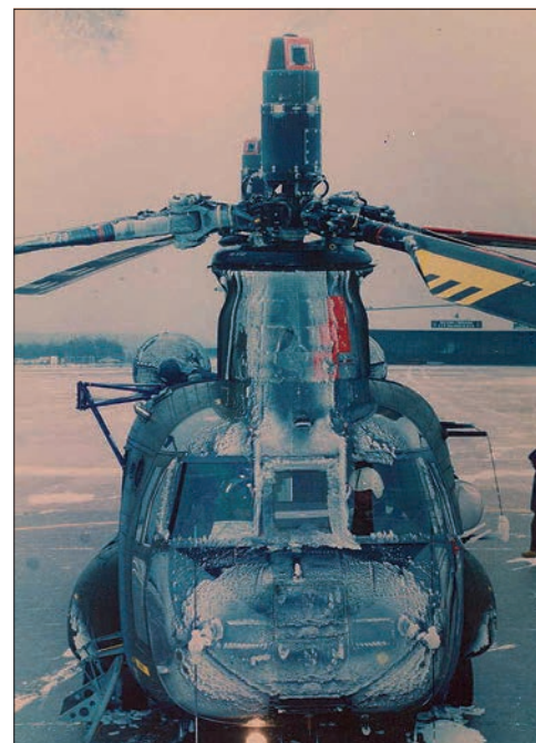
The Chinook after the flight in freezing rain over Prince Edward Island, with the record-breaking amount of ice on it
