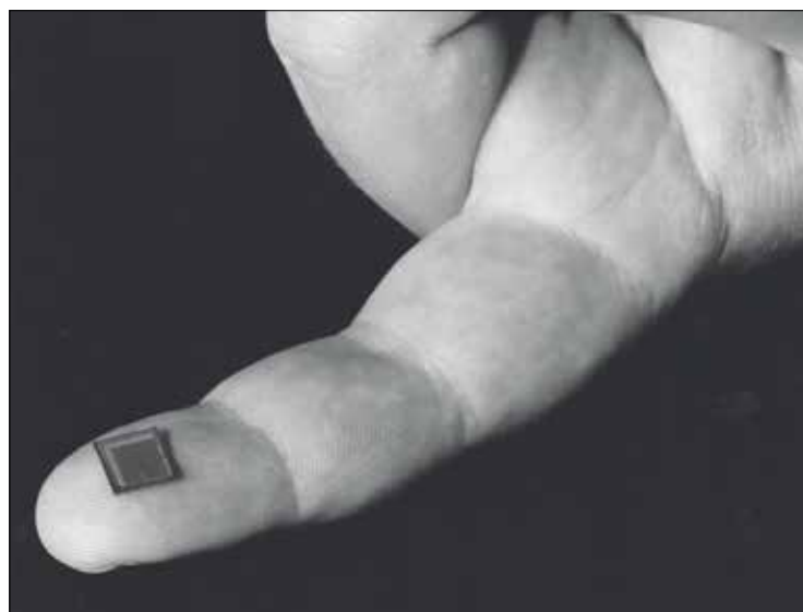
CMOS sensors paved the way for smaller cameras and the development of the 'camera on a chip'. Although not as high quality as CCD sensors, they use less power and are cheaper to produce. They are also integrated into fingerprint recognition on smartphones and are used for identification in biometric passport booths for border control
