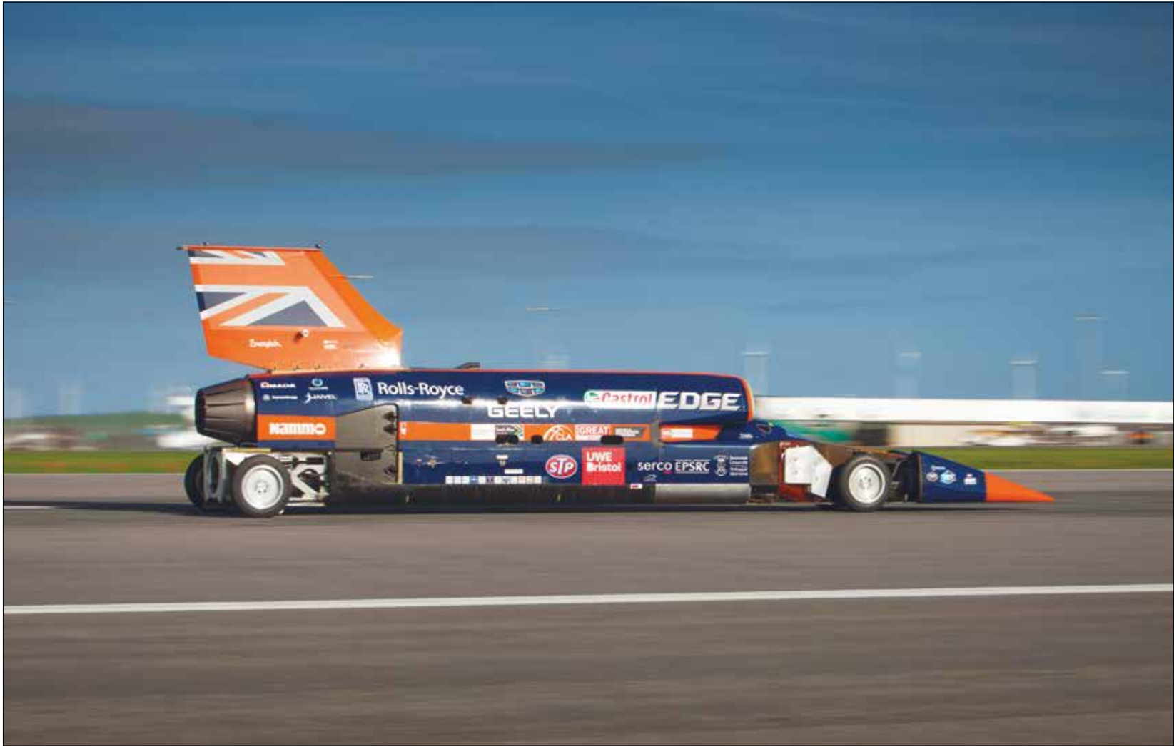
The Bloodhound Supersonic Car reached speeds of 320 kph during testing at Cornwall Airport Newquay in October 2017. The tests have set in motion the process for the car's land speed world record attempt in South Africa in 2018 © Stefan Marjoram
