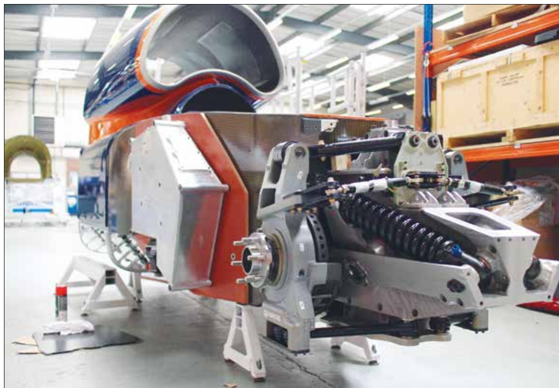
The Bloodhound's steering suspension joint is split and truncated, and the two parts move independently of each other. This gives the best suspension stiffness and prevents the wheel from flexing off line, which can cause instability © Stefan Marjoram
