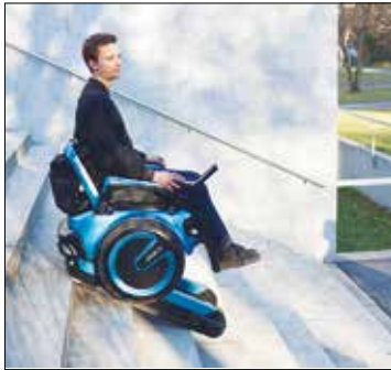
The Sewco wheelchair is just one innovation on display at the Beazley Designs of the Year Exhibition. The wheelchair's set of retractable tracks allow users to travel up and down steps without assistance
