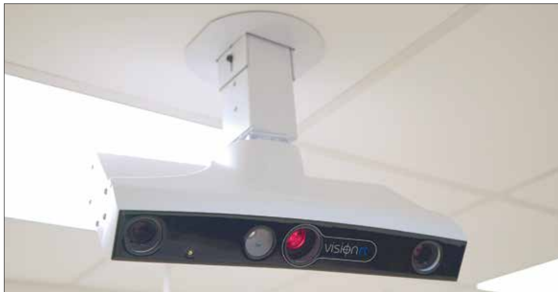
Each of the ceiling-mounted modules contain a projector and stereoscopic camera. These need to be precisely aligned and rigid
