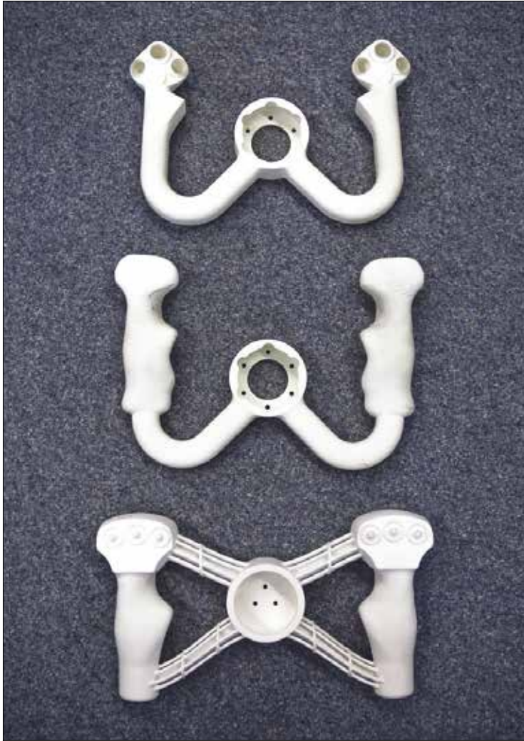
Prototypes of the Bloodhound's steering wheel were 3D printed using moulds of driver Andy Green's grip. The final design (bottom) was 3D printed in titanium by Renishaw © Stefan Marjoram
