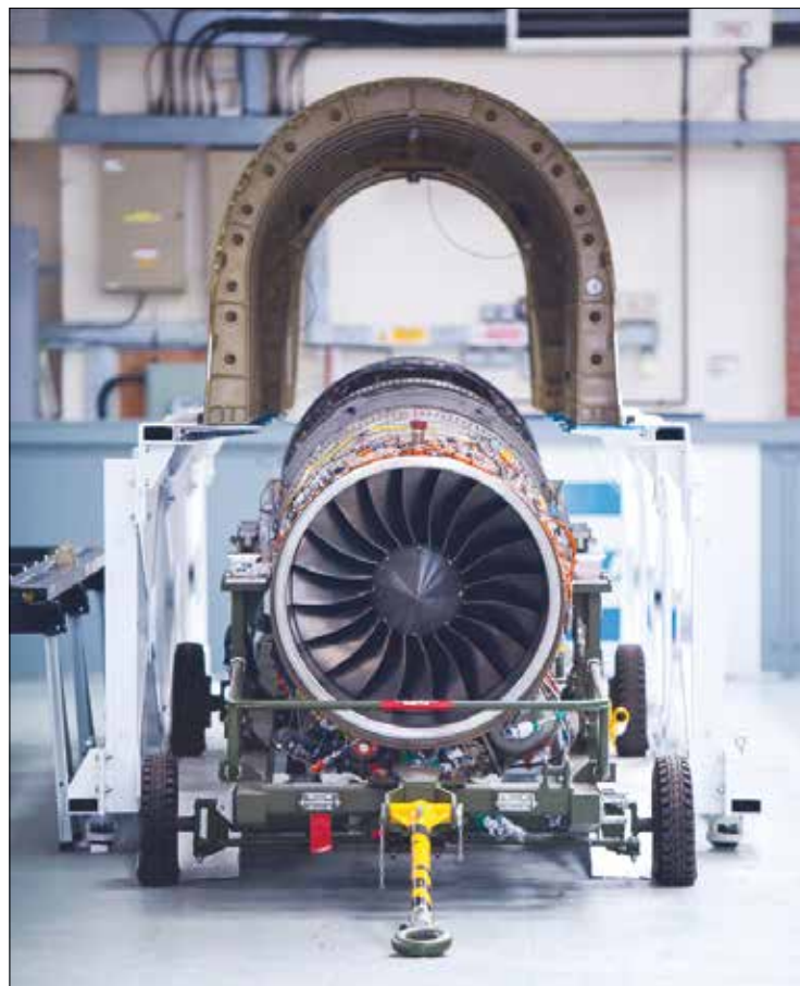
The Bloodhound was fitted with a jet engine designed for use in military fighter aircraft. This proved to be something of a challenge and resulted in changes to the shape of the car © Stefan Marjoram
