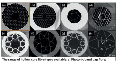
The range of hollow core fibre types available: a) Photonic band gap fibre; b to h) Various anti-resonant fibre designs (reproduced from Poletti F (2014) 'Nested antiresonant nodeless hollow core fiber', *Opt. Express 22*, 23807-23828)
