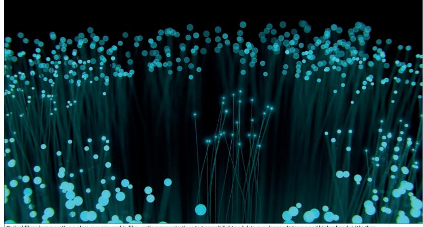
Optical fibres incorporating a glass core are used in fibre-optic communications to transmit light and data over longer distances and higher bandwidths than electrical cables. A new generation of hollow core fibres is being developed to transmit data more efficiently © Joshua Kimsey/Pixabay
