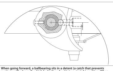
motion until released), which locks the wheel into a straight position. When enough lateral force is applied, the wheel can twist away from that detent position and steer. The twisting force necessary will be different for each person so an especially designed adjustable spring was made and the detent shaped to control the way the ball moves away from its locked position © Trekinetic
