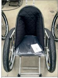
The Hyperforma seat insert was originally invented by an occupational therapist and is filled with tiny polystyrene balls. Once the wheelchair user is in position, a hand pump is applied to a valve under the seat, air is expelled and the resulting vacuum makes the balls stay in their pre-set position © Trekinetic
