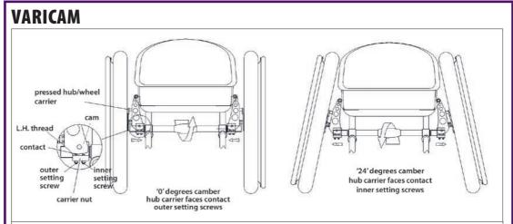
Diagrams show the mechanism that enables users to reangle their wheelchair's wheel © Trekinetic
