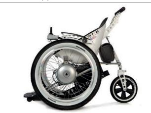
Trekinetic's powered GTE wheelchair, which has just three components and can easily be folded to fit in the boot of most medium-sized cars © Trekinetic
