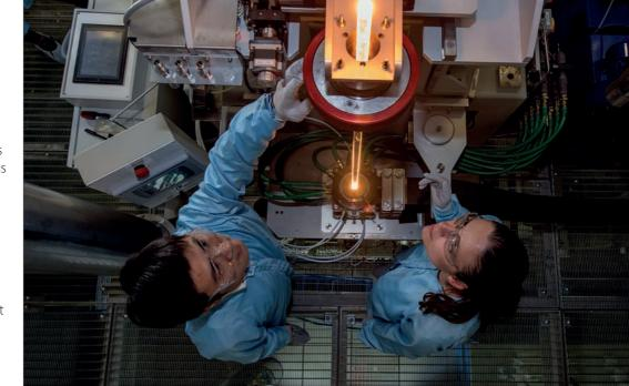
A fibre preform being fed into the furnace at the top of the fibre optic draw down at the Optoelectronics Research Centre fibre optic draw tower
