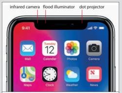
The iPhone X's 3D facial recognition technology projects over 30,000 dots onto a user's face to map their features and uses the information to unlock the phone in the future. The dots are invisible to the human eye but can be seen through an infrared camera, which captures the image and sends the data for confirmation. The flood illuminator is an invisible infrared light that identifies facial features even when it's dark © Apple
