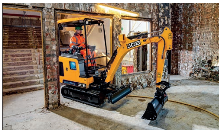
The innovative fully electric digger, 19C-1E, developed by JCB © JCB
