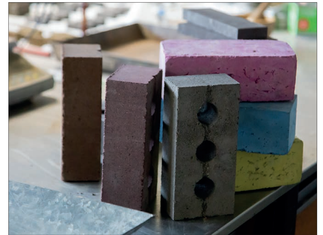
K-briqs can be made in a range of colours by adding recycled pigments to the mix
