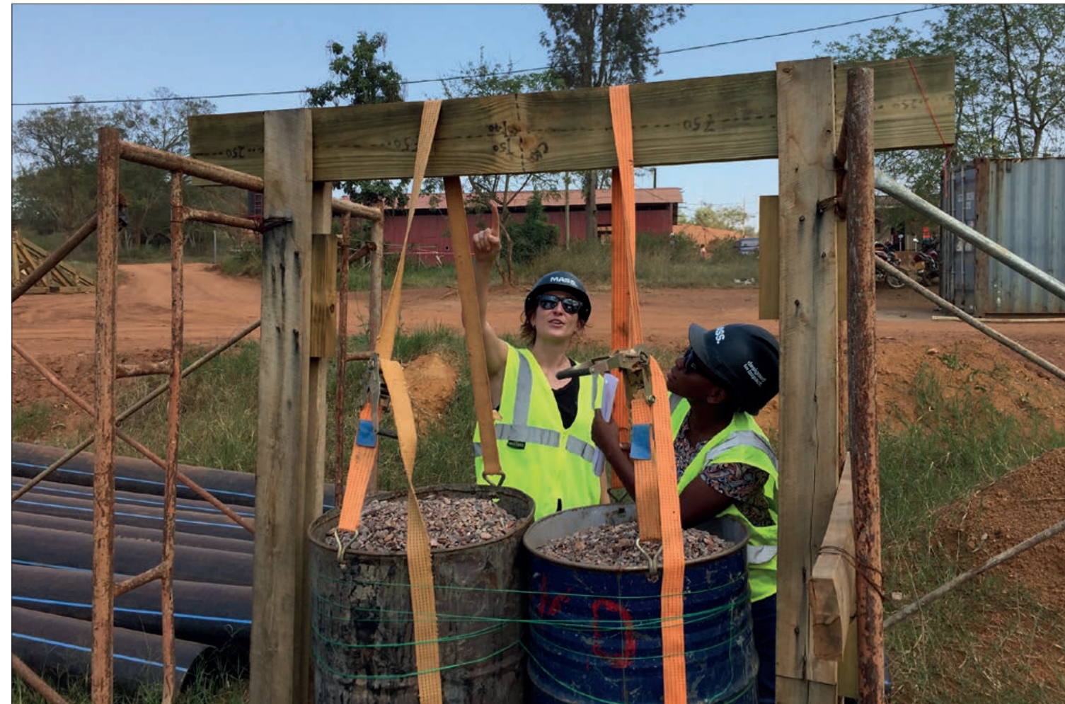
Rosie and Shakira load testing a timber beam with buckets of stone
