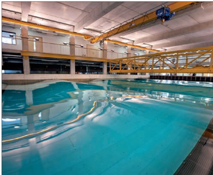
COAST's ocean basin can generate waves and currents to enable testing of new energy technologies © COAST, University of Plymouth
