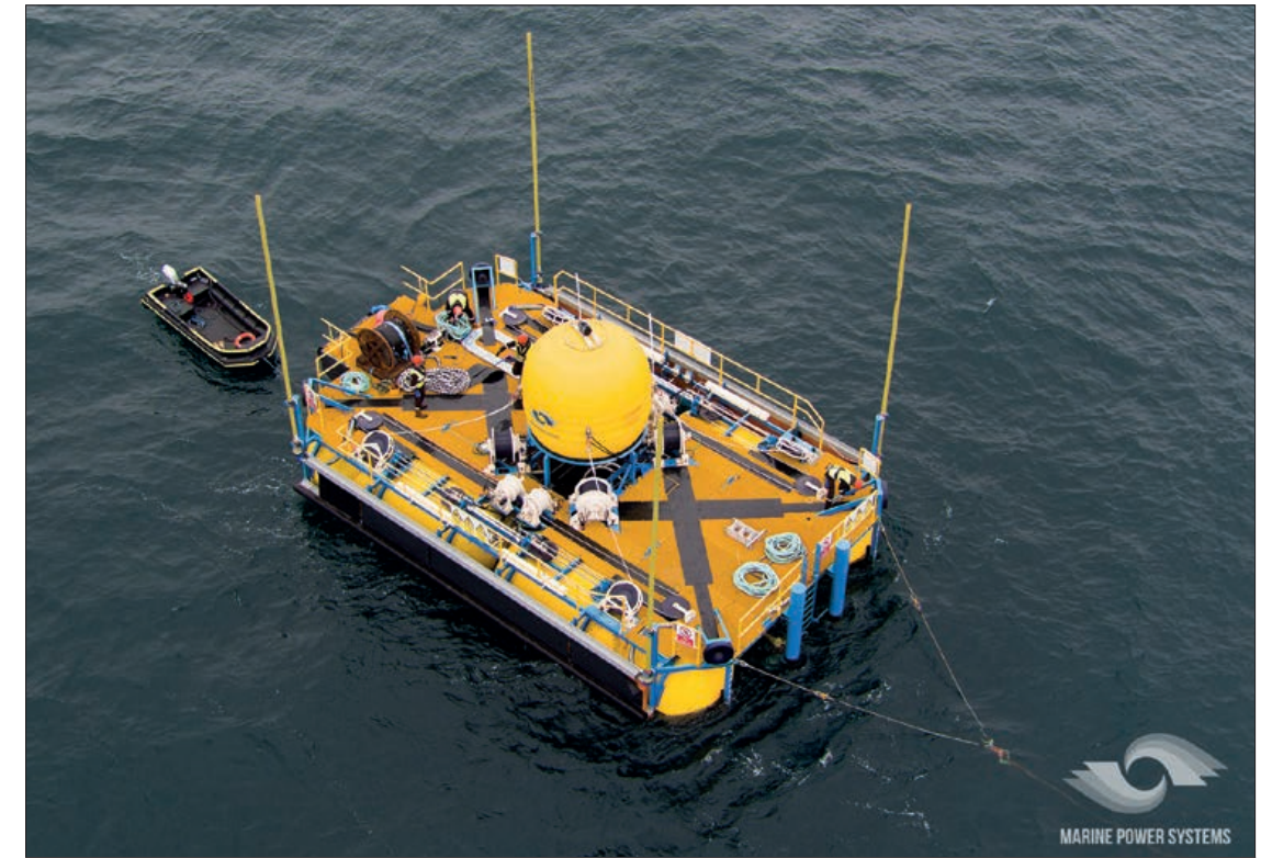
WaveSub harnesses the motion of sub-surface water particles © Marine Power Systems
