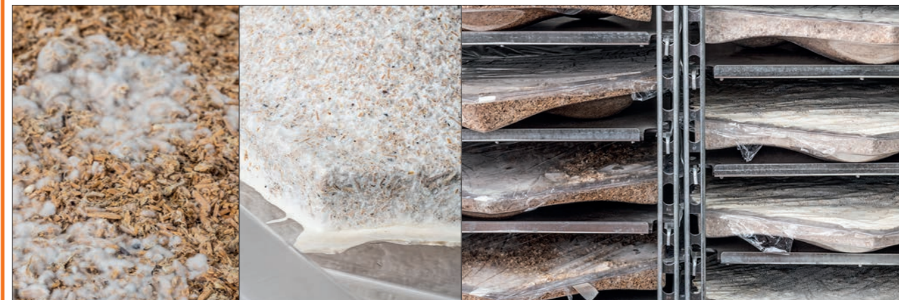
Growing a tile. (Left) The mycelium begins to grow on the substrate. (Centre) A denser mat of mycelium. (Right) The tiles before and after growth © Mogu
