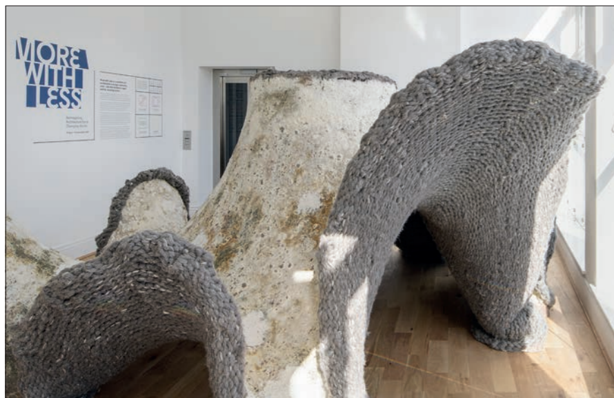
The Hub for Biotechnology in the Built Environment's knitted mycelium structure, 'grown' from local waste materials at the Farrell Centre in Newcastle © Jill Tate
