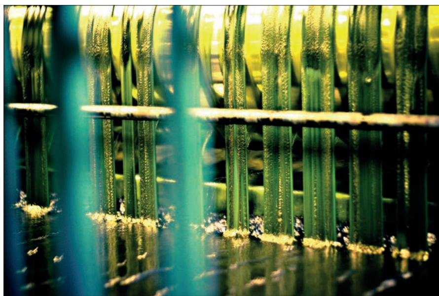
The rope dyeing process, where yarns are bundled before going through the dye bath © ORTA
