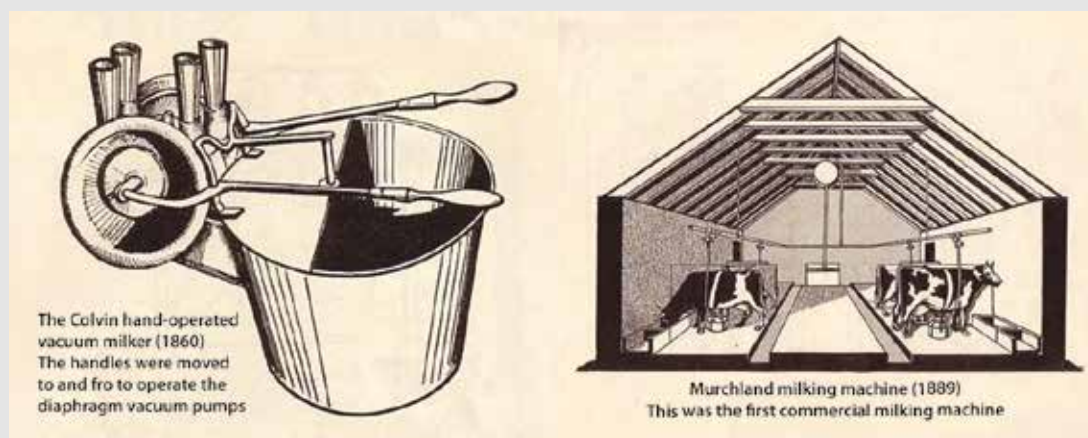
Although not robotic, innovative engineering was employed in the Colvin hand-operated vacuum milker in 1860 (left) and the first commercial milking machine developed by Murchland in 1889 (right) © Fullwood
