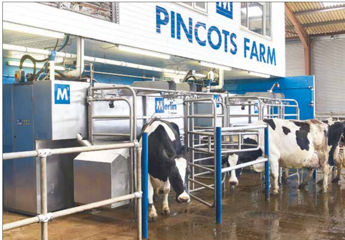
Cows are encouraged into the automated milking stall by a feeding trough at one end. The rear gate closes when the animal's presence is detected by a photocell, which also records the cow's identity via an electronic tag © Fullwood
