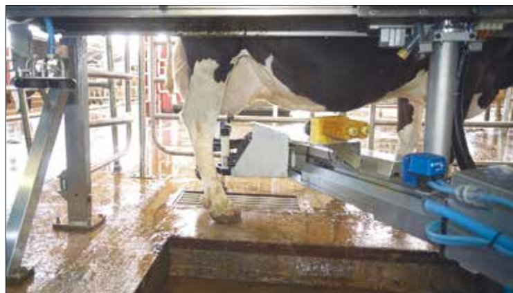
A robotic arm in the milking stall uses stored coordinates to locate the position of the cow's teats, which are then washed by soft brushes on the arm. A laser tracking system is then also employed to improve more accurate positioning of the suction cups © Fullwood
