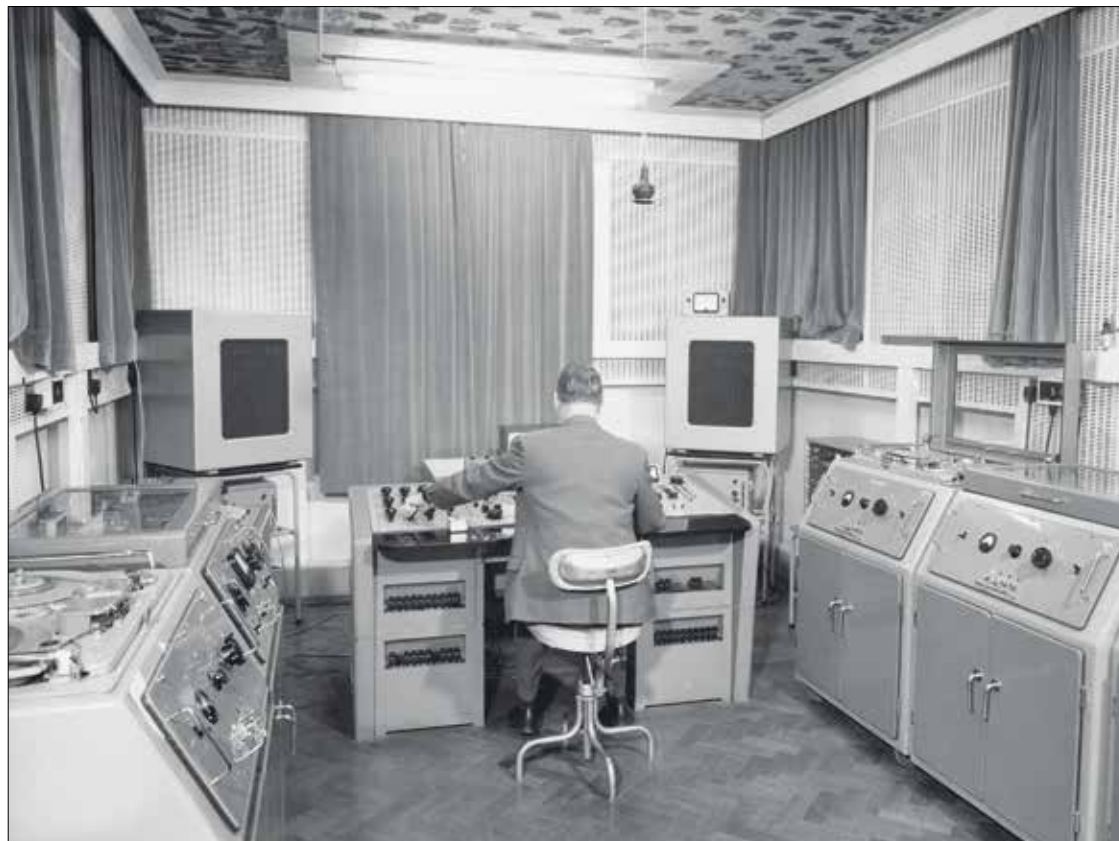
Engineer Gus Cook works with BTR-3 tape machines, one of which was rediscovered at the University of Southampton in 2016, in room 11 at Abbey Road Studios around 1965 © Abbey Road Studios
