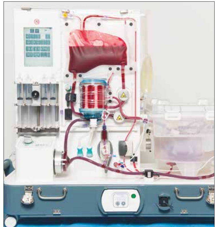
The OrganOx metra can store a functioning liver at body temperature for 24 hours, allowing longer time for a suitable patient to be matched
