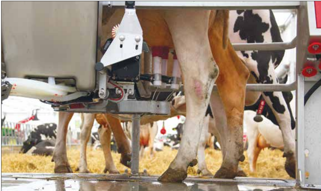
A liquid flow sensor in the system that is electrochemically activated by milk can tell whether the cup is attached incorrectly and when the milk production has ceased, automatically allowing the suction cups to be removed. Inbuilt instrumentation can also run checks on the milk's quality and quantity © Royal Association of British Dairy Farmers
