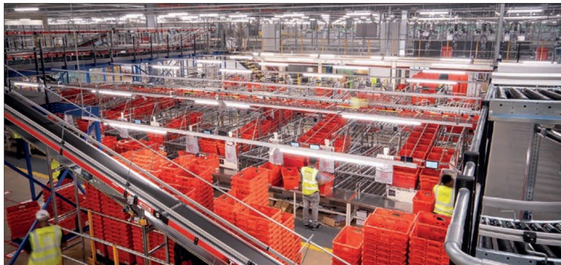
At any one time, there are around 8,000 plastic crates on the move across 32 kilometres of conveyor. Over 150,000 orders per week are dispatched from this warehouse © Ocado
