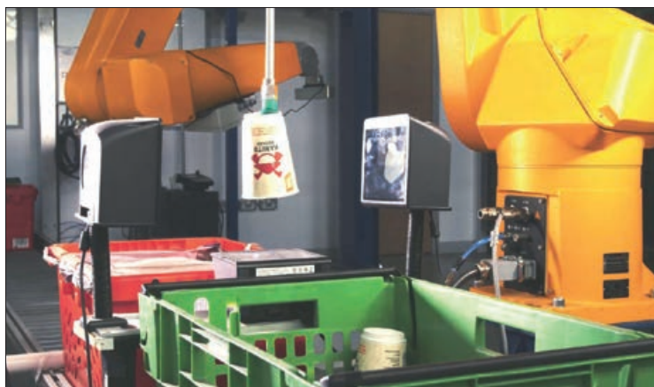
Ocado's robotic picking system uses a suction cup attached to an articulated arm. This is guided by a computerised 3D vision system that calculates grasping points on an object regardless of its shape and deformability © Ocado
