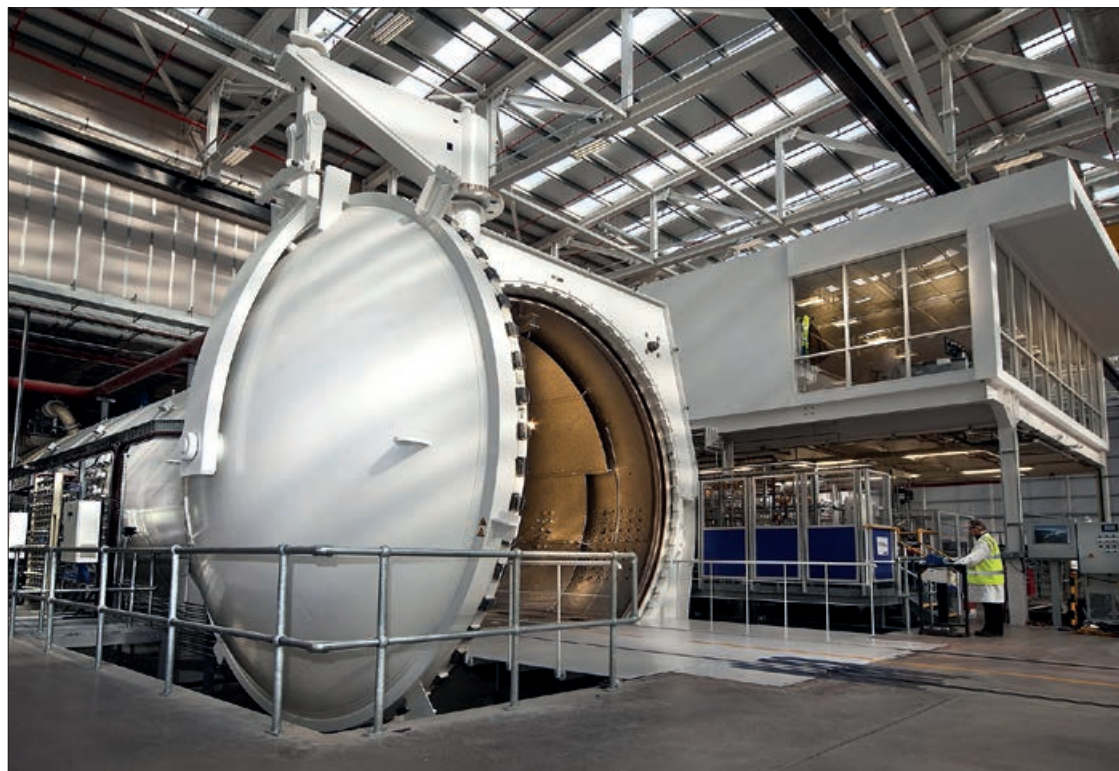
The autoclave area in the Wing Manufacturing and Assembly Facility at Bombardier Belfast where the wings are cured © Bombardier
