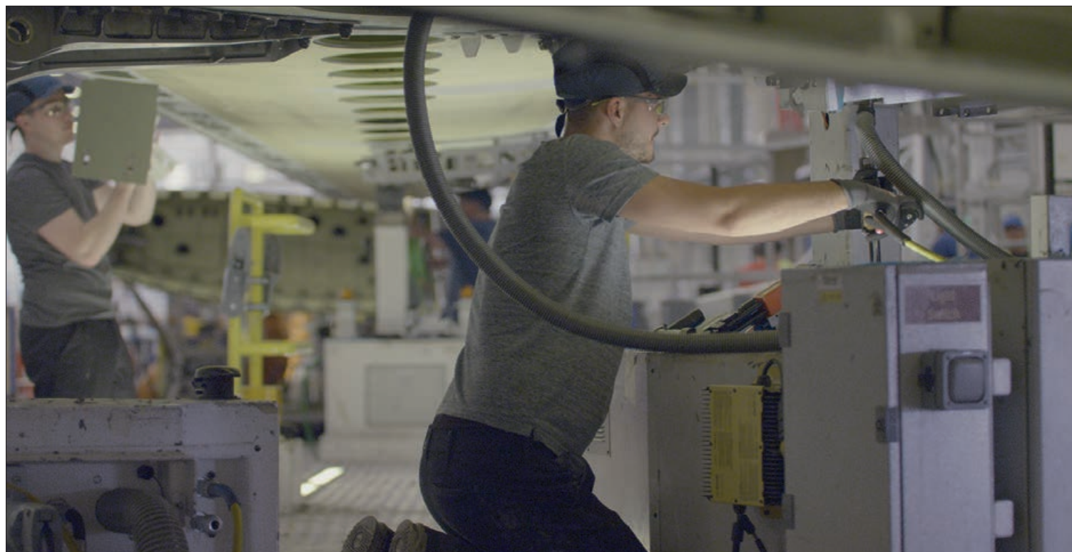
Bombardier aircraft fitters work on kitting out the wing in final assembly before despatch © Bombardier
