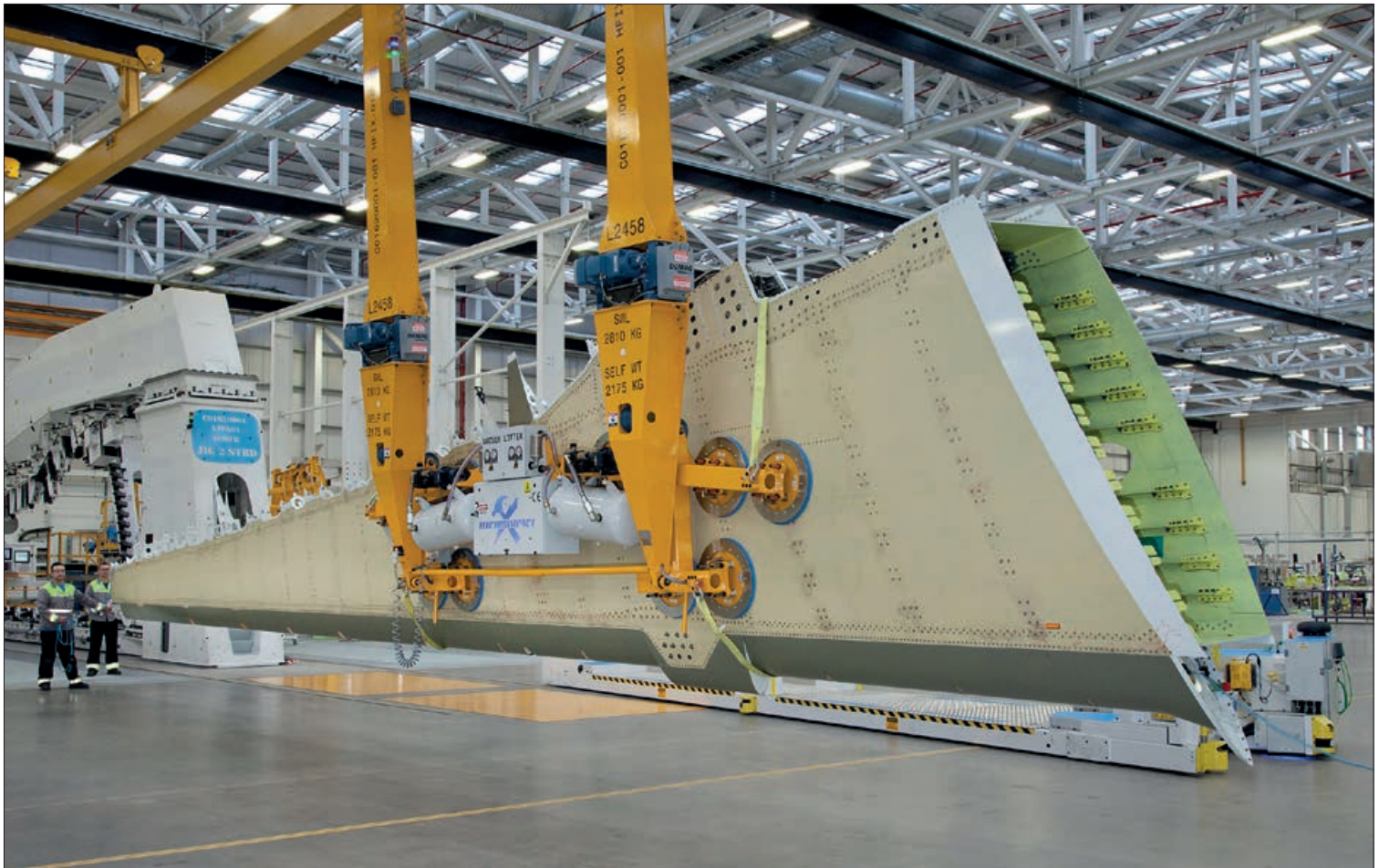
An advanced composite wing being lifted from a jig in final assembly © Bombardier
