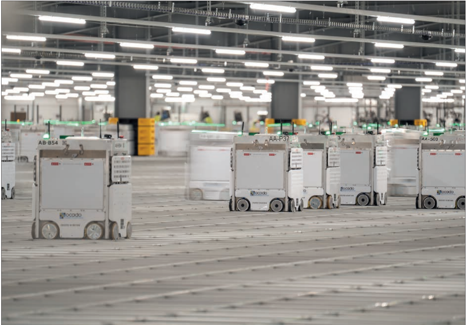
Bots whizz around the two grids at Erith, each the size of three football pitches and holding nearly up to 3,500 bots © Ocado
