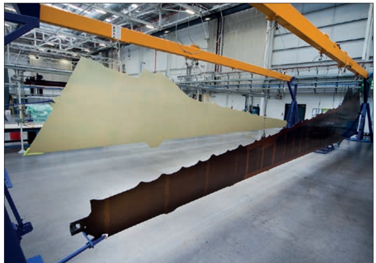
A one piece A220 wing skin produced by the RTI process © Bombardier
