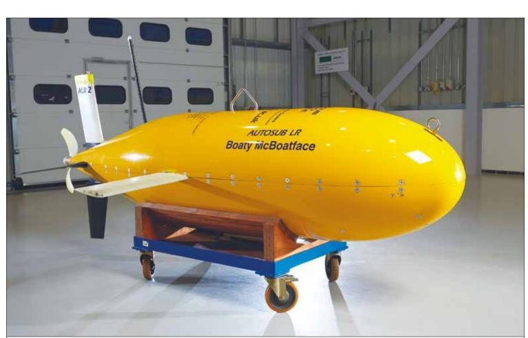
Boaty McBoatface is one of several autonomous unmanned vehicles onboard the RRS Sir David Attenborough. Robotic submarines and marine gliders will collect data on ocean conditions and marine biology and deliver it to scientists working in the ship's onboard laboratories © National Oceanography Centre
