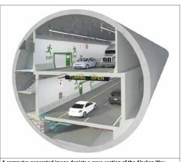
A computer-generated image depicts a cross-section of the Alaskan Way tunnel, showing four lanes of highway with with two at the top and two at the bottom © Washington State Department of Transportation
