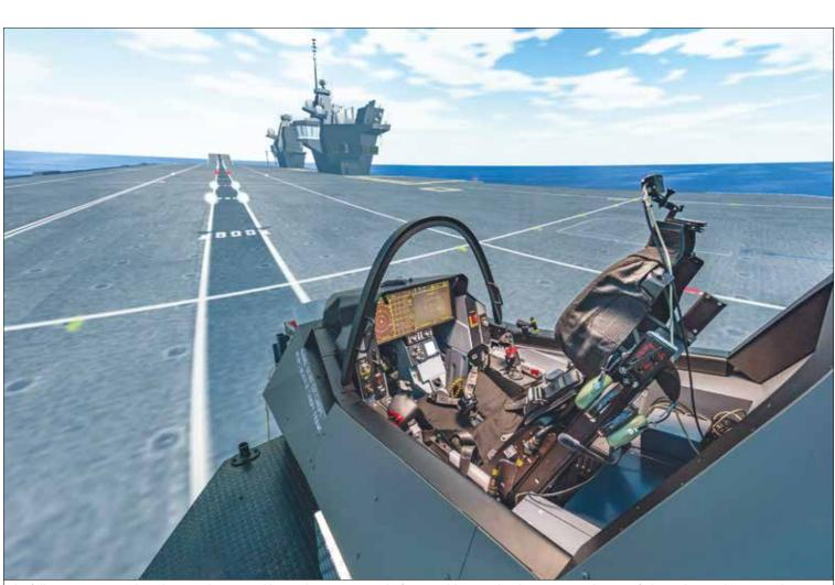
The fully immersive simulator has a cockpit moved by an electric motion platform. Highly specialised engineering data was fed into the simulator to replicate the disturbances that an aircraft would experience, meaning that when a pilot lands an F-35 in the simulator, they feel the motions that they would feel in real life © BAE Systems
