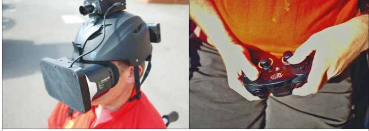
lan wearing his helmet with a modified webcam (left) that is controlled by a wireless PlayStation controller (right)
