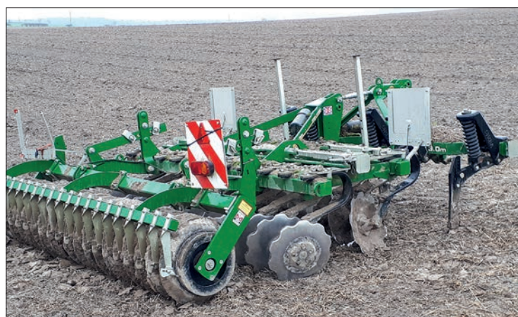
Discs and tines are designed to cultivate only a narrow seedbed so that buried soil carbon is not exposed to the atmosphere, which causes CO 2 emissions
