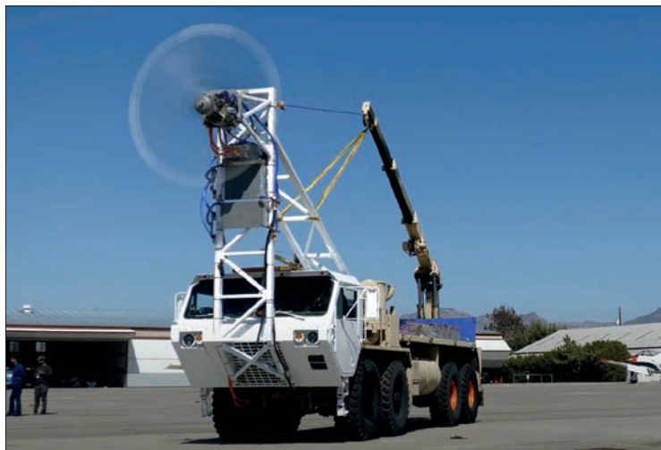
In August 2021, ZeroAvia's hydrogen powertrain successfully pulled a 15 tonne HyperTruck mobile ground testing platform across the tarmac. The HyperTruck is based on heavy-duty military trucks and is sized for the company's ZA-2000 2 MW+ powertrain, which can be used to test systems for 40- to 80-seat hydrogen-electric powered aircraft
