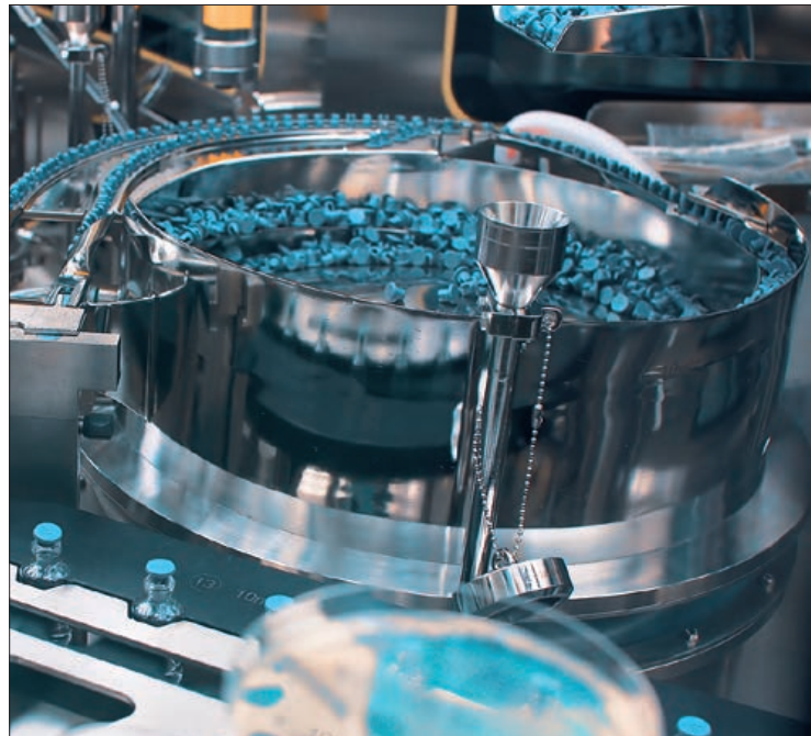
Vaccine manufacture will consist of automatic packaging machines such as this for packaging ampoules with vaccine, injection and medical drugs © Shutterstock
