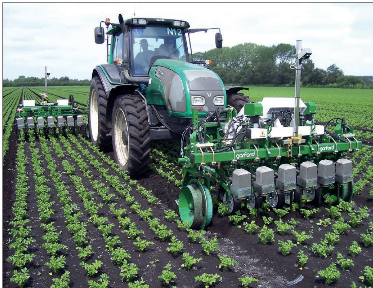
A Garford Robocrop in-row automatic hoe system operating with two-metre wide sections – these are matched to the width of the drill or transplanter
