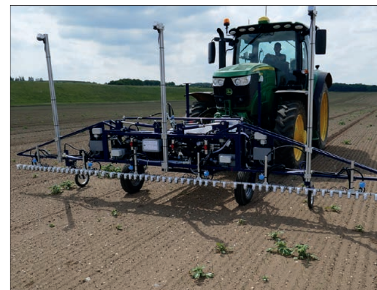
A spot sprayer working in a crop of onions to treat volunteer potatoes – a difficult weed in this crop. The tractor is steered with GPS but the vision system positions the spray nozzles relative to the crop
