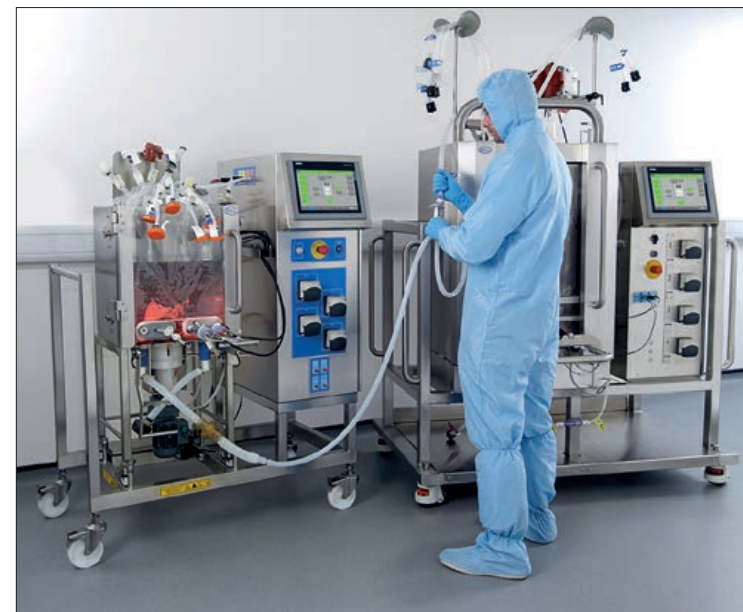
Bioreactors are an example of the specialist manufacturing equipment the VMIC has purchased for its virtual VMIC facility, such as these Allegro™ STR bioreactors 50 L and 200 L © Pall Corporation
