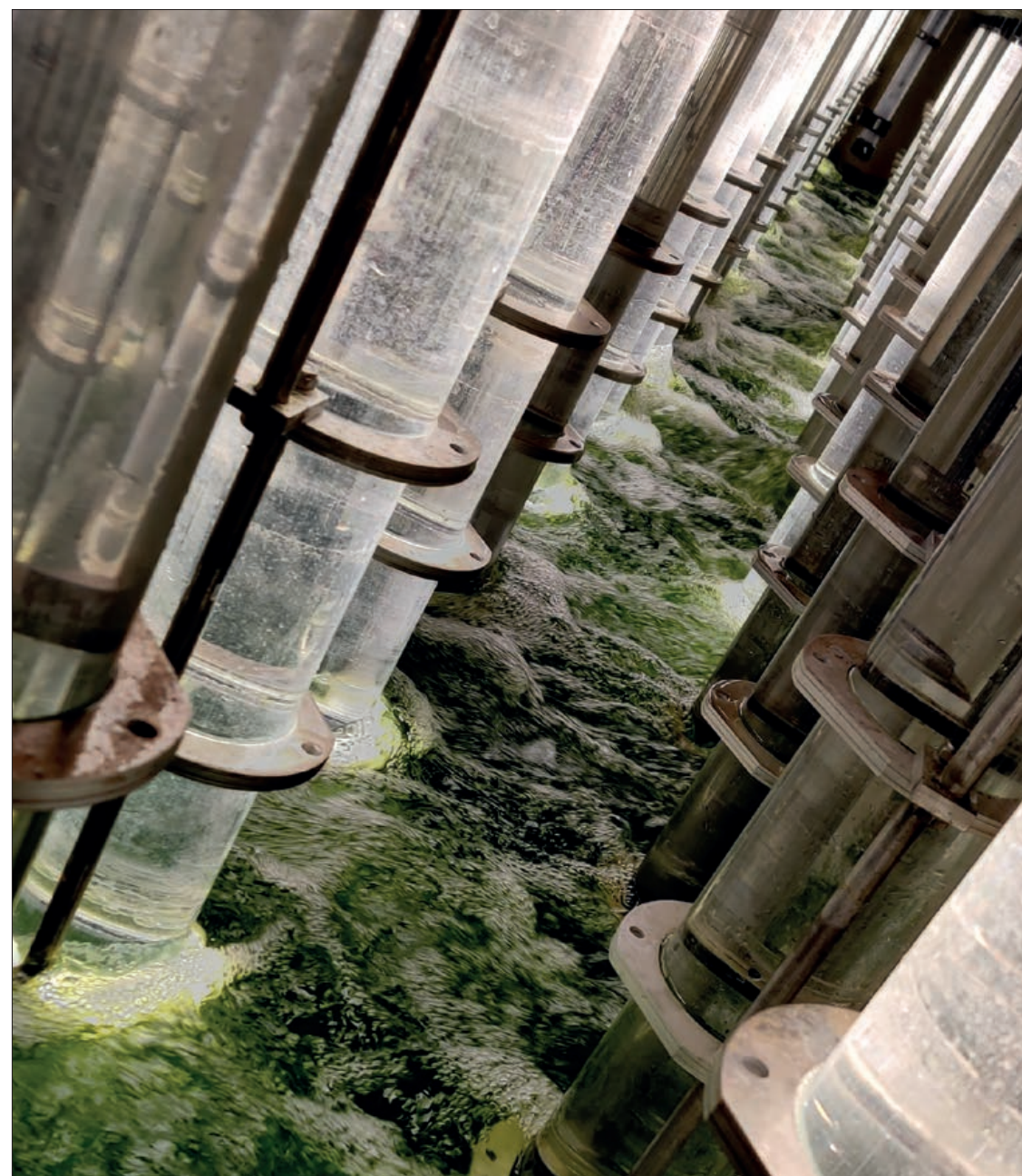
Algae is used in wastewater tanks to purify the water © I-Phyc
