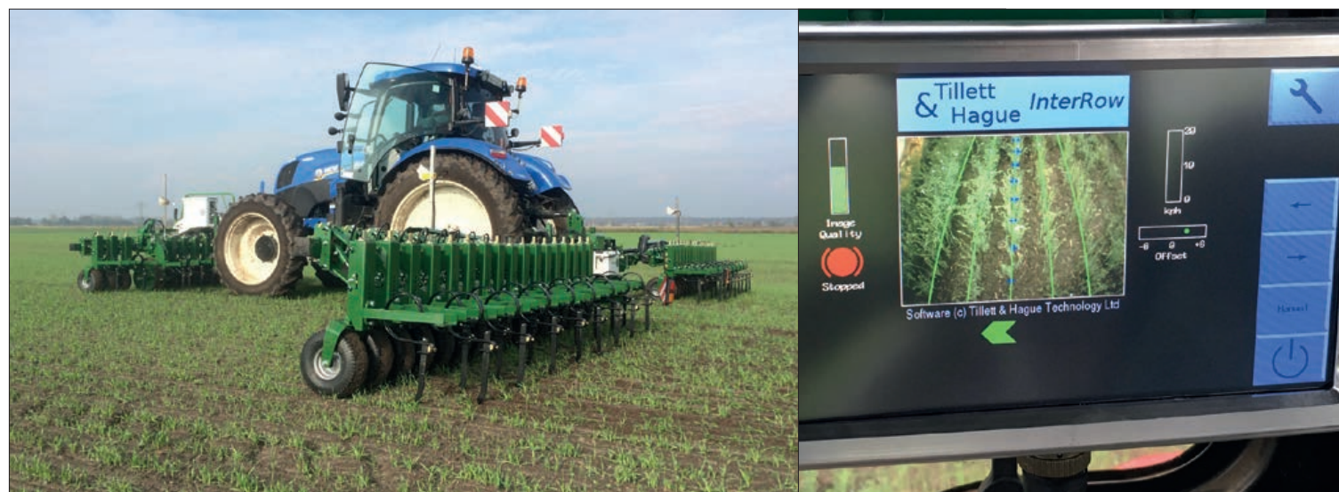
Three tractor-mounted 6-metre wide sections of vision-guided hoe and (inset) the control and monitoring system for the machine
