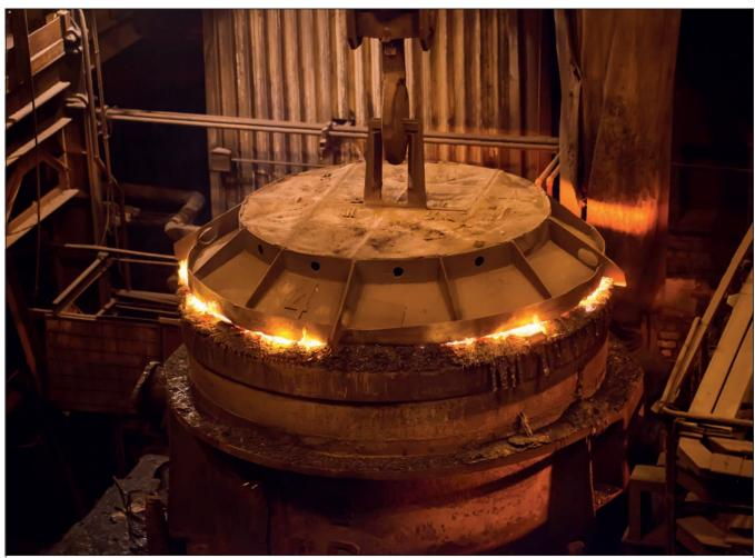
An electric arc furnace. Its characteristic domed roof is closed over the bowl-shaped hearth. Electrodes protruding from the roof are melting scrap steel inside © Shutterstock
