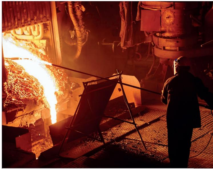
A steelworker tapping a molten sample from the blast furnace to test its composition © Shutterstock
