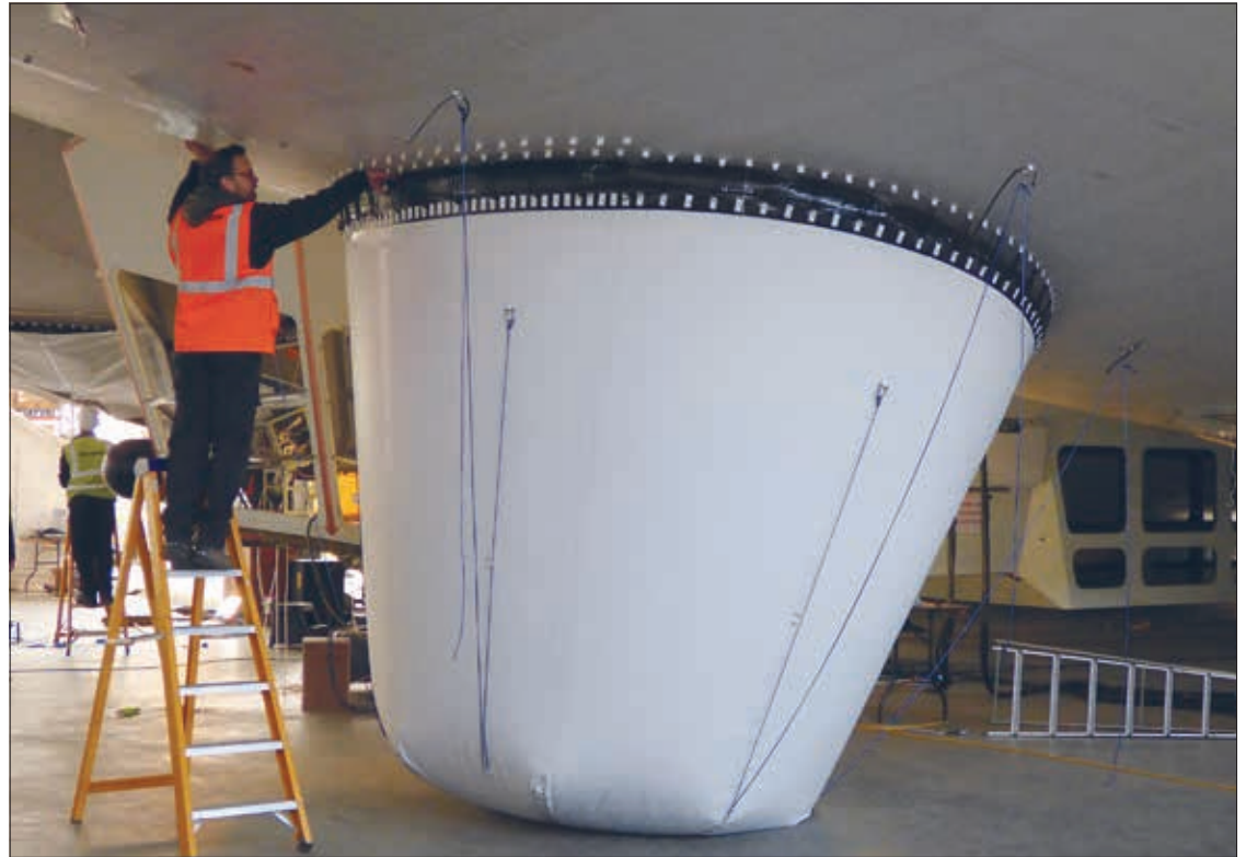
The auxiliary landing system was added to the craft following its crash. The system, a pilot-deployable two airbag landing system that acts as an extra cushion to land on, allows the aircraft to land safely at a greater range of landing angles. The airbags are over three metres in length and contain 15 cubic metres of gas (less than 0.1% of the entire hull volume) and are situated on each side of the flight deck to offer enhanced protection to the cabin and flight deck. The system uses the existing ballonnet fans to inflate, and takes under 20 seconds to be ready for use © Hybrid Air Vehicles
