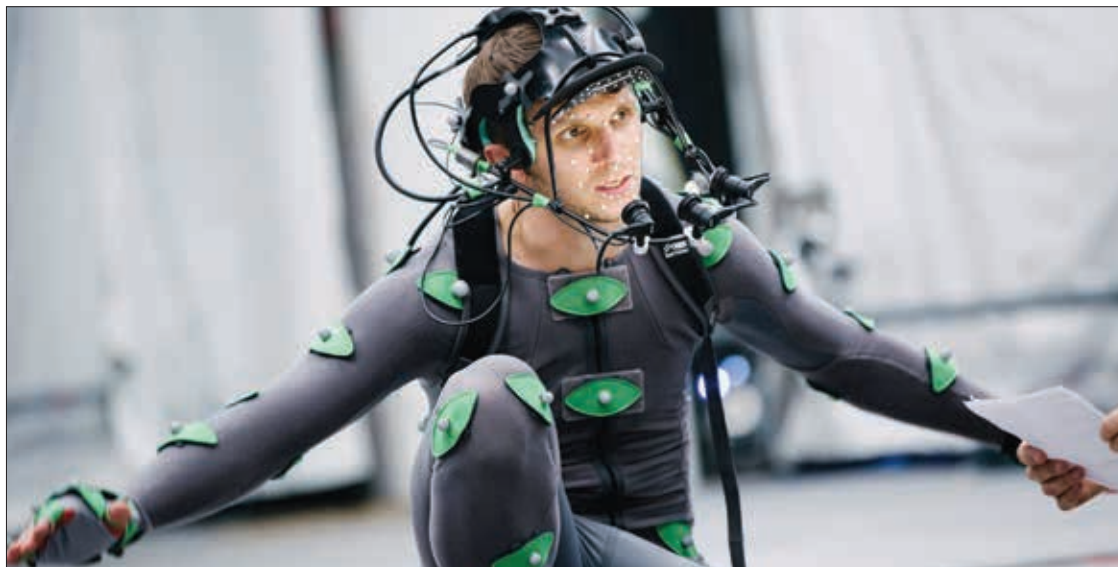
Motion capture technology involves actors wearing suits covered in reflective markers that pick up their movements
