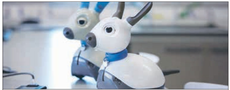
One of the robots to be showcased at Robotics Week is MiRo, a fully programmable autonomous platform that is suited to developing companion robot animals © UK-RAS
