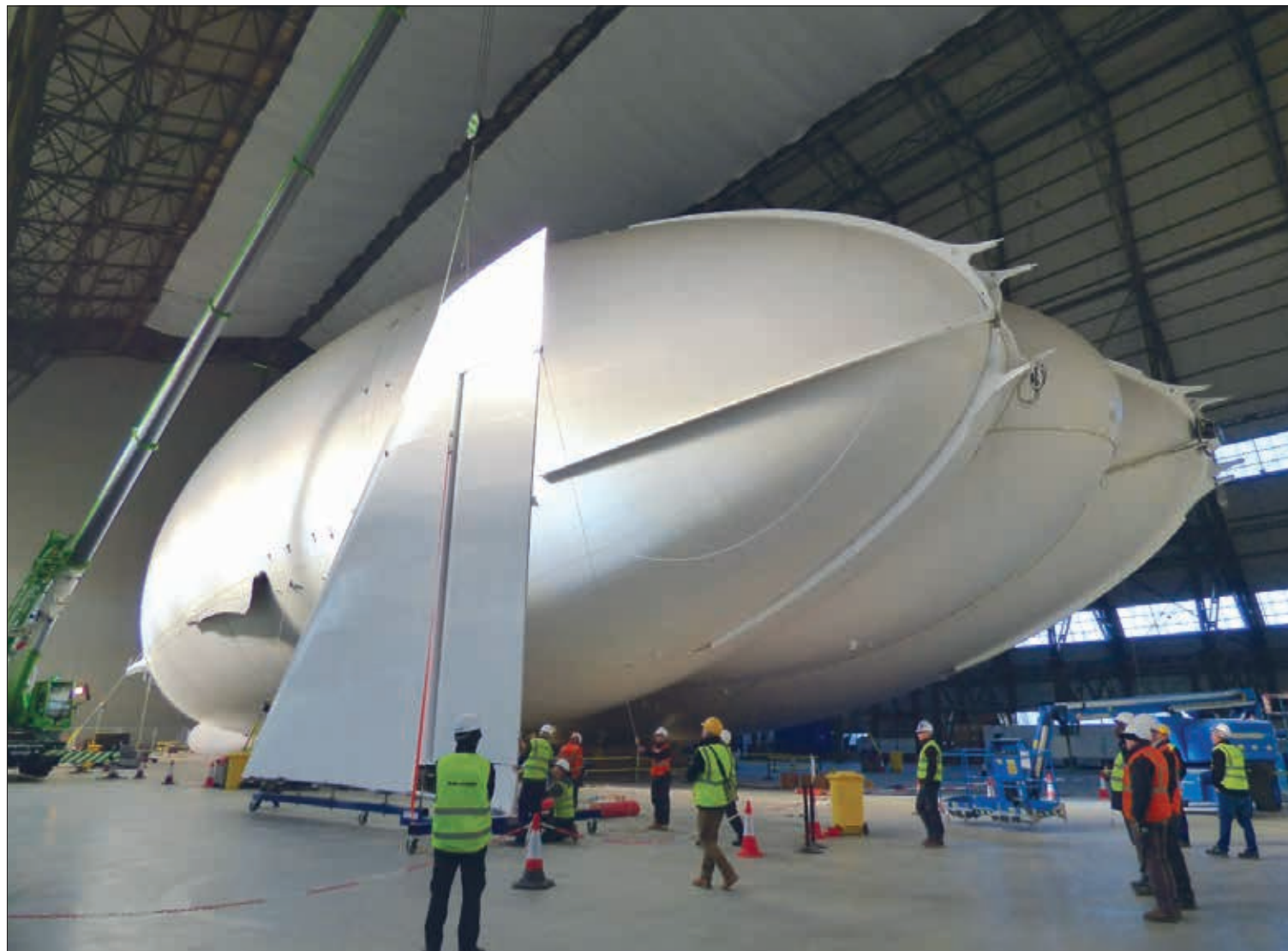
From the back, the Airlander resembles three sausages that have been squashed together, an arrangement that creates an aerodynamic shape, which is assisted by two top fins and two lower fins – one of which can be seen before it was attached to the hull © Hybrid Air Vehicles
