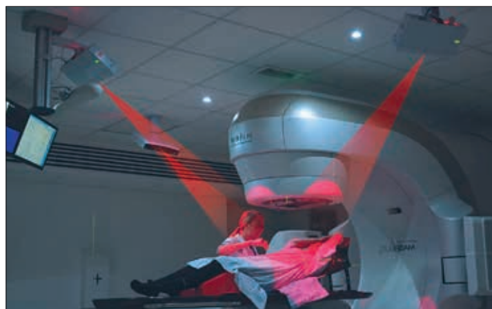
Ceiling-mounted AlignRT camera units map the surface of a patient's body to ensure that radiotherapy beams are correctly delivered and paused if the patient makes any slight movement © Vision RT
