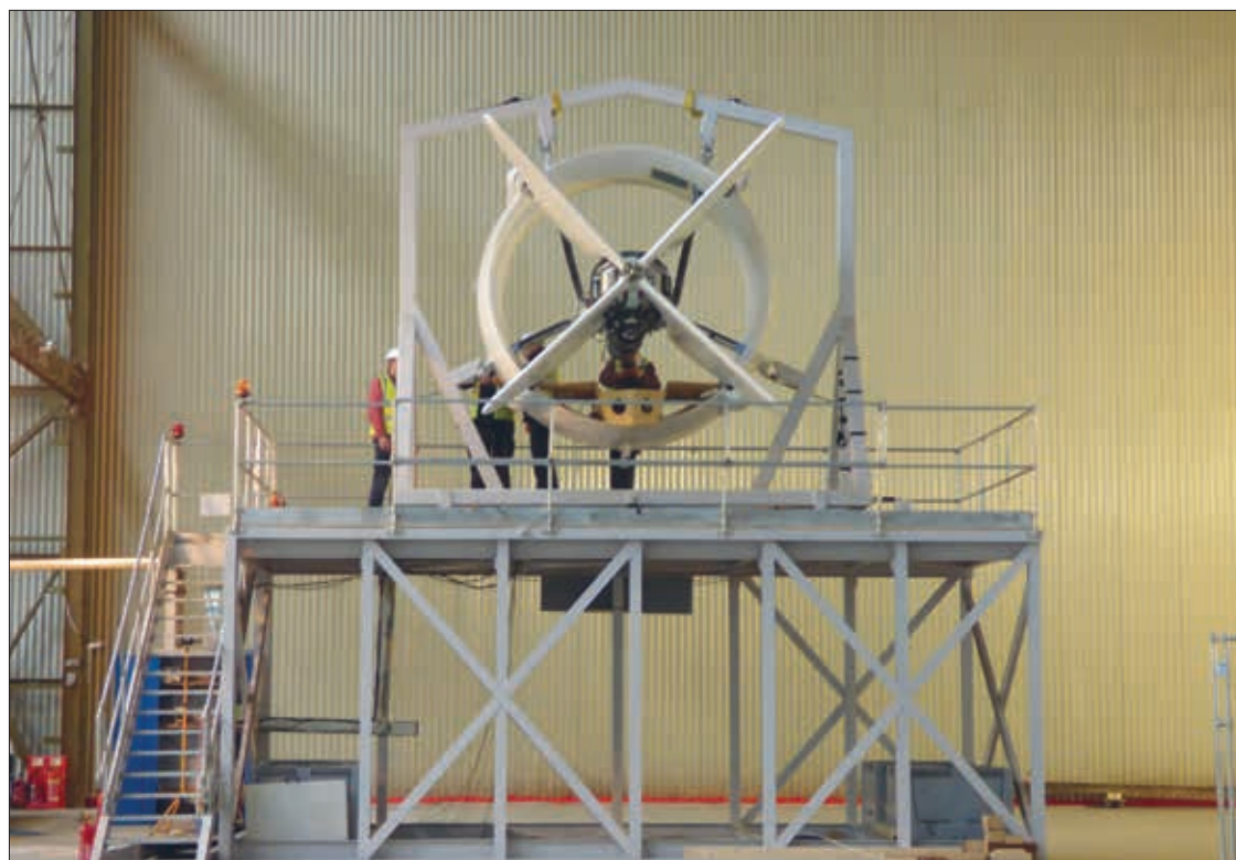
Four 325 horsepower turbocharged engines with variable pitch propellers power the Airlander. They are lighter than engines that were used for previous generations of airships and the absence of a rigid interior framework means that they need to be attached directly to the fabric structure of the craft © Hybrid Air Vehicles
