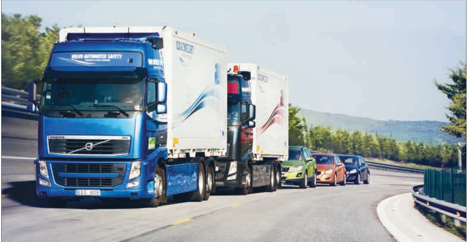
Professor Jackson believes that platooning, where automated heavy goods vehicles follow each other under the guidance of the lead vehicle, could make this form of transportation more energy efficient and transform drivers' working hours © Ricardo
