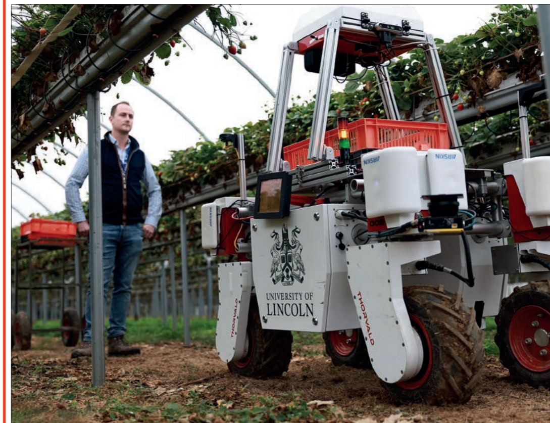
The University of Lincoln's Thorvald robots are equipped with LiDAR (light detection and ranging) sensors and cameras that enable them to comprehend their immediate surroundings. This helps when meeting human pickers who have summoned them to transport their fruit or if they unexpectedly meet humans who have come across their path, ensuring that the robots don't impact or get too close to them © University of Lincoln
