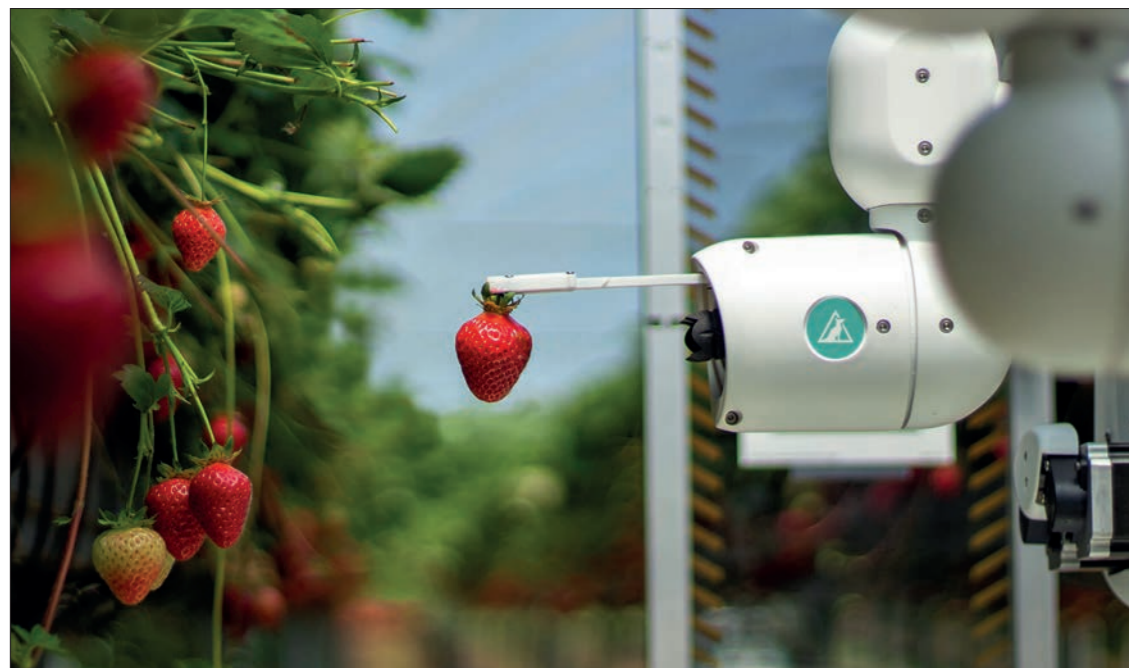
Dogtooth's picking device comprises a pair of slender grippers and resembles a pair of tweezers. A separate cutting edge extends forward and cuts the stalk above the grippers leaving them holding the single strawberry by its stalk. The robot arm then carries the fruit to a quality control system where it is analysed for any defects before being placed into a punnet or waste chute © Dogtooth
