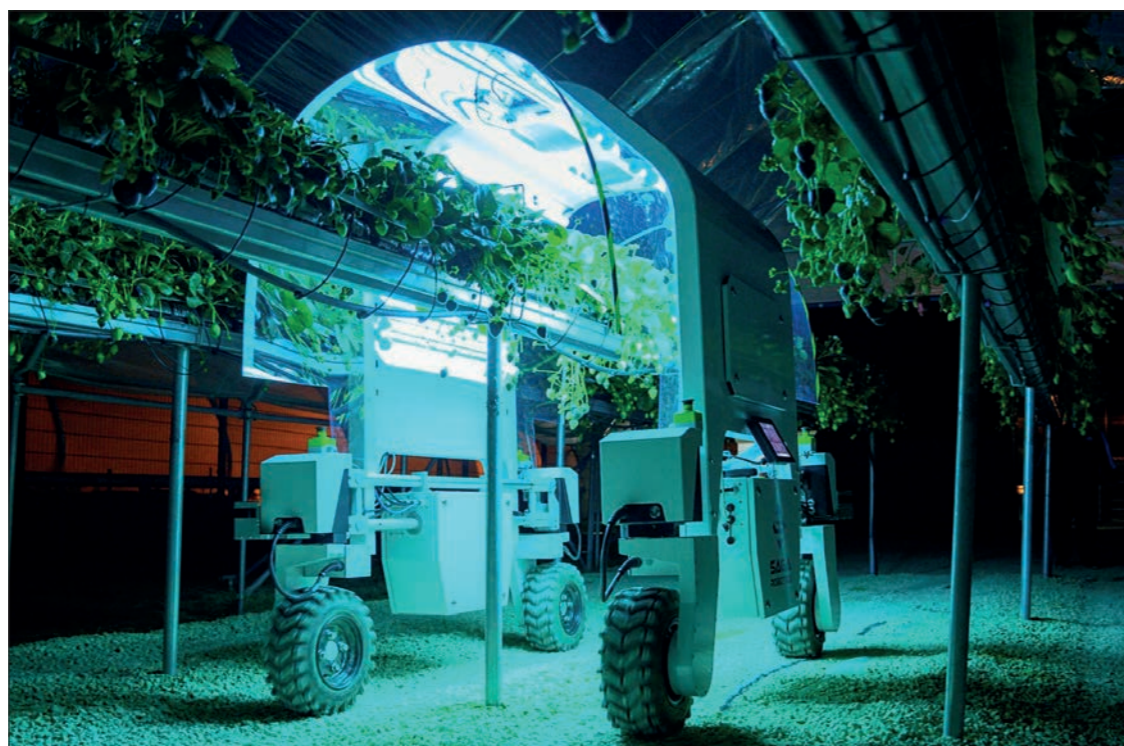
Saga autonomous robots apply shortwave light to strawberry plants to prevent powdery mildew © Saga
