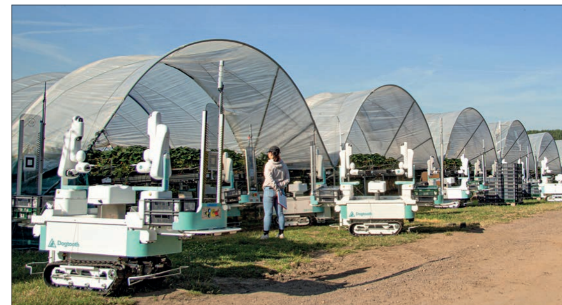
Horticultural autonomous robots need to be built to withstand mud, rain, dry bumpy ground, and dust for hours at a time © Dogtooth
