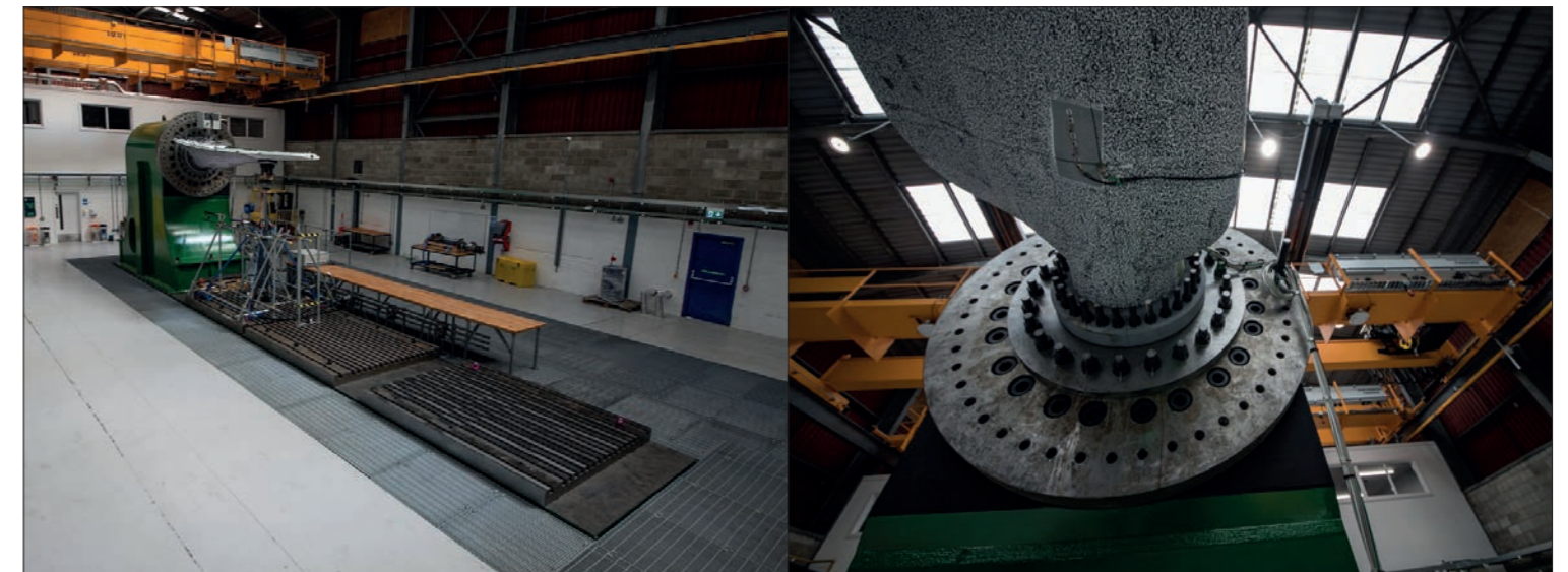
(Left) The FastBlade system in action, with a tidal blade in place, ready to be tested. (Right) A close up of the speckle pattern applied onto the blade's surface © FastBlade
