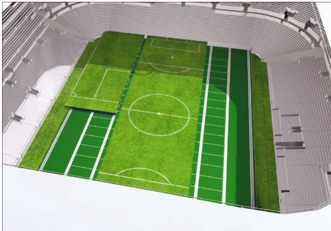
A computer-generated image shows how the three trays carrying the pitch will slide over the artificial NFL field below © Tottenham Hotspur / SCX Special Projects
