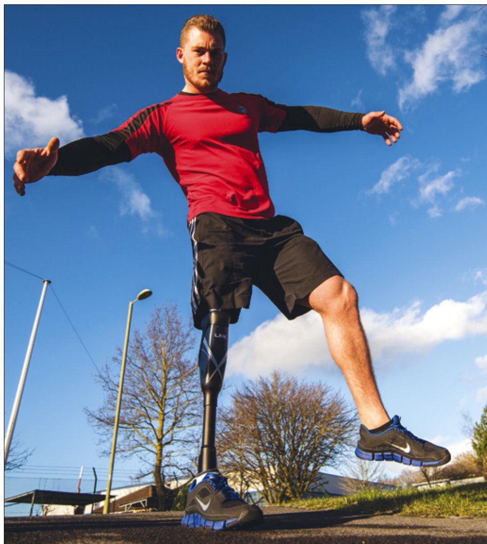
The 2016 MacRobert Award-winning Linx limb system, developed by Blatchford, is the first ever prosthetic limb with integrated robotic control of the knee and foot, in which the sensors work together so that users can walk, balance and be supported on all types of terrain © Blatchford
